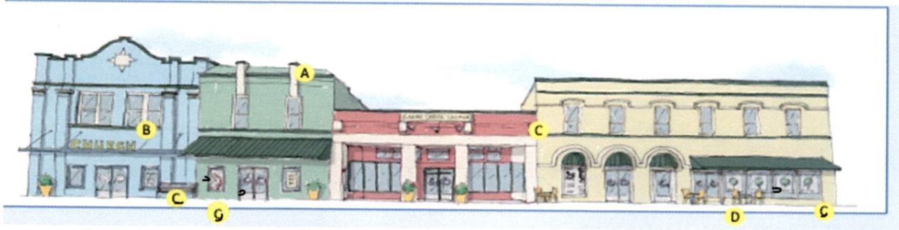
Sample Façade Articulation Elements: Example B: A=Cornice, B=Spandrel Panel, C=Parapet, D=Pedestrian amenities, E=Window signs. Source: Downtown Wharton Master Plan 2024.
