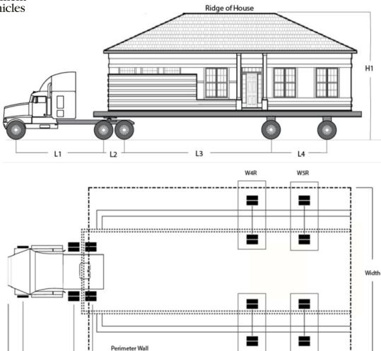
The diagrams above are examples. Please report your axle configuration exactly as your load is configured to include any extra axles that are not depicted above. Axle Spacings (Example: L1 to L2, L2 to L3...) and weights per axle (Example: W1, W2, W3...) must be documented in the chart below.
