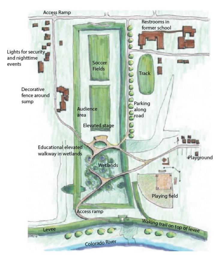
The proposed sump areas for the levee project might include a number of minor modifications to allow for community enhancements yet still maintain the full design and functionality of retaining floodwater. (Drawing by Paula Loomis, PhD, AICP, FAIA, LEED AP)
