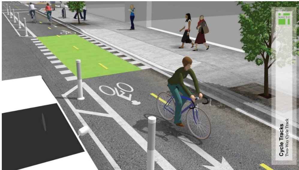
This rendering from the NACTO Urban Bikeway Design Guide depicts a cycle track. This on-street protected facility offers a high-quality result for a small investment.
